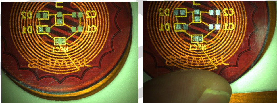
Figure 4: J.A.M.E.S Coin before and after cleaning
