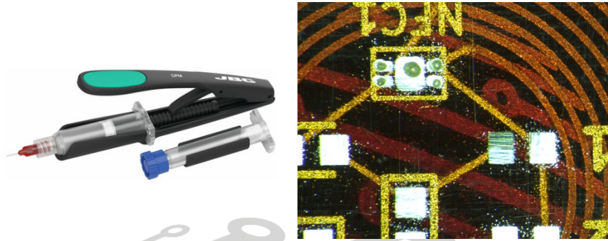
Figure 3: Use of a manual dispenser for placing H20E paste (here on the Pads of NFC Tag component)
