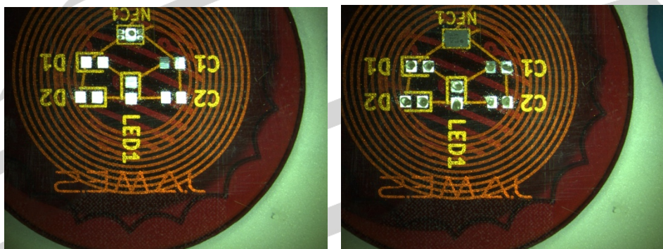
Figure 4: Manual dispensing of H20E paste
